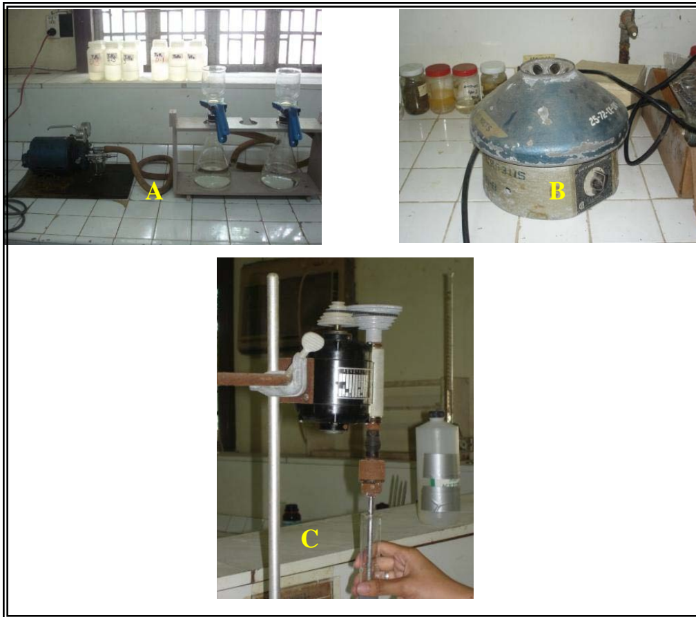
Figure 6. The millipore filter apparatus (A), the centrifuge (B) and the homogenizer (C)
