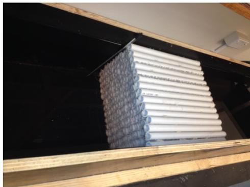
*Figure 3. Flow Straightener*
