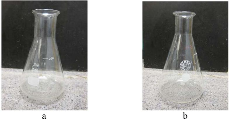
Figure 4. Flasks used for measurements of retention times: (a) 330 ml flask with 4 cm diameter mouth; (b) 630 ml flask with 4 cm diameter.
